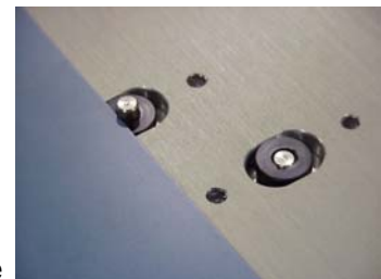
With PLC controlled stops registration is transferred automatically and accurately.
